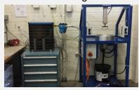
This equipment reduces repetitive motion and ergonomic strain to the employees by eliminating the manual method of packing grease into the wheel bearing. We completed this task more efficiently, saving production man-hours.
